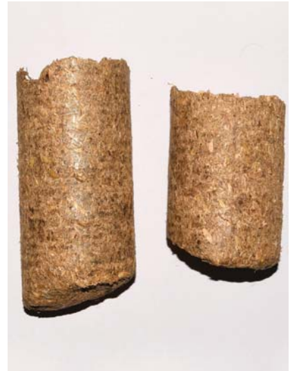
Figure 3: Binder-less briquettes of chopped paddy straw
